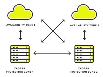
With Zadara Multi-Zone HA, Virtual Private Storage Arrays are constructed from resources that are distributed between different protection zones, located in separate physical facilities within the same metropolitan area. In the event that one of the protection zones becomes unreachable, for instance due to network or power failure or localized flooding, VPSA failover is initiated and the resources in the surviving protection zone take control and provide uninterrupted access to data.
